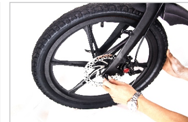
Step 4: Tighten the bottom bracket screw of the left side front fork, should not screw too tightly.
