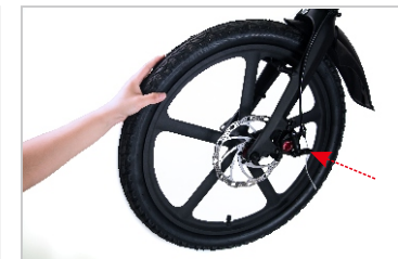
Step 6: Rotate the front wheel, if there is no friction, it is fixing. Or trim the screw on the brake until there is no friction.
