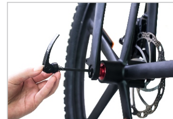
Step 3: Insert the axis from the right side, for each side of the bottom bracket , there is a small spring, and the spring circle towards inside.
